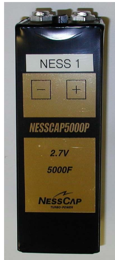
Fig. 6. Double layer capacitor 5000 F Nesscap.
